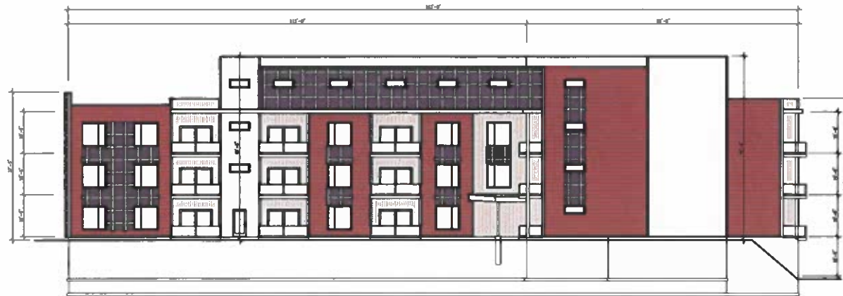
② APARTMENT BUILDING - EAST ELEVATION SCALE: 1/8" = 1'-0"
