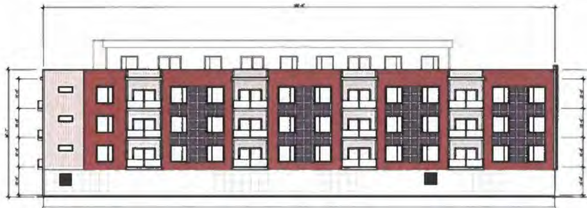
① APARTMENT BUILDING - WEST ELEVATION SCALE: 1/32" = 1'-0"
