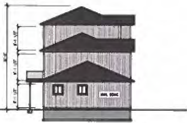
④ TOWNHOUSE - NORTH ELEVATION SCALE: 3/32" = 1'-0"
