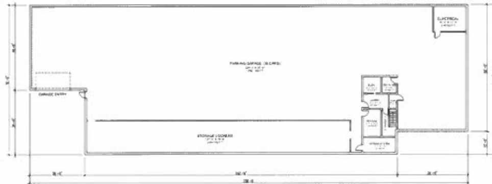
1 LEVEL-0 FLOOR PLAN SCALE: 1/16"=1'-0" FLOOR AREA 16,365 S.F. 39 VEHICLE PARKING SPACES
