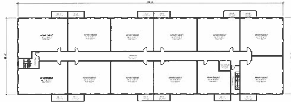
3 LEVEL-2, 3, 4 FLOOR PLAN SCALE: 1/16"=1'-0" FLOOR AREA 15,048 S.F. 12 APARTMENTS
