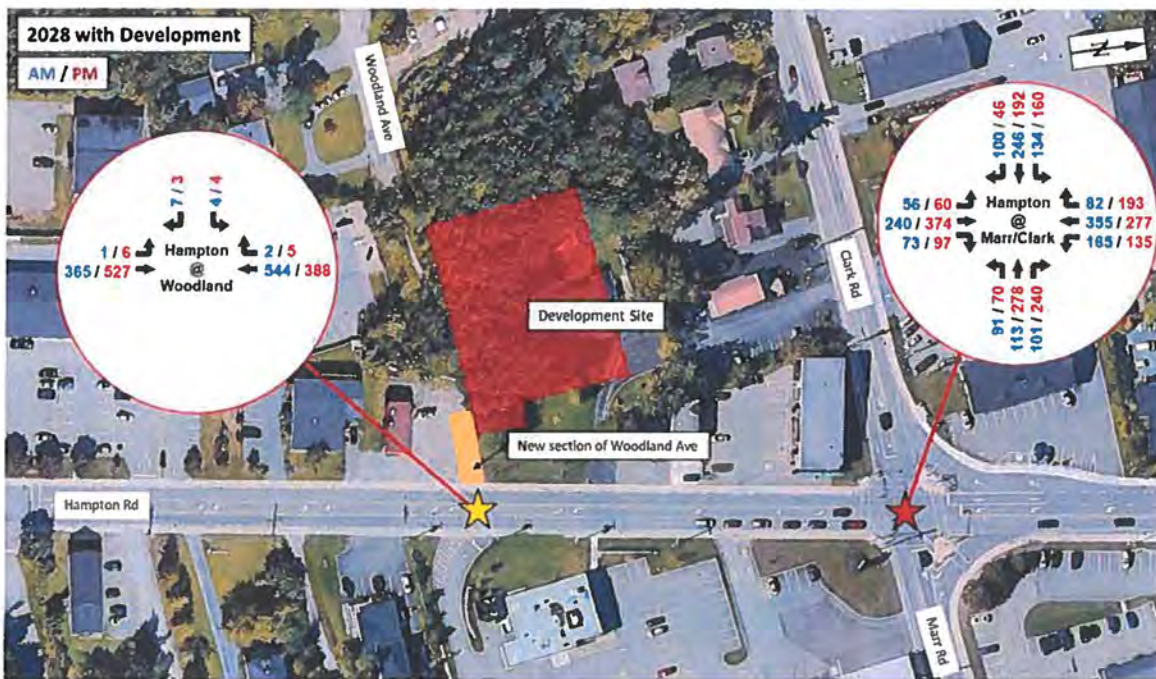
Figure 2 – 2028 Traffic Volumes with Development Traffic
