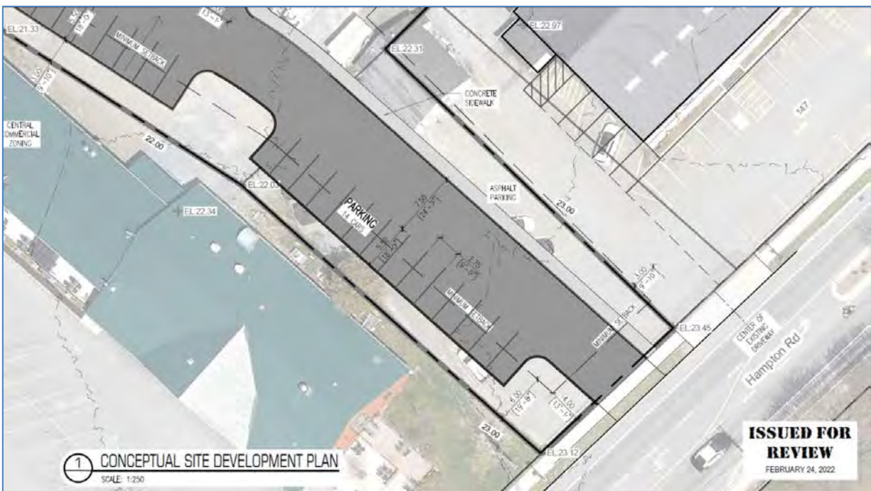
Figure 4 - Revised Driveway Entrance with Separation from 147 Hampton Road
