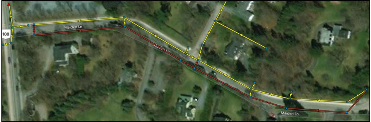
Figure 6-1: Proposed Maiden Lane Sewer Upgrade Concept (proposed sewers in red)
