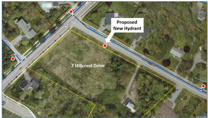
Figure 2 - Proposed New Hydrant Location
