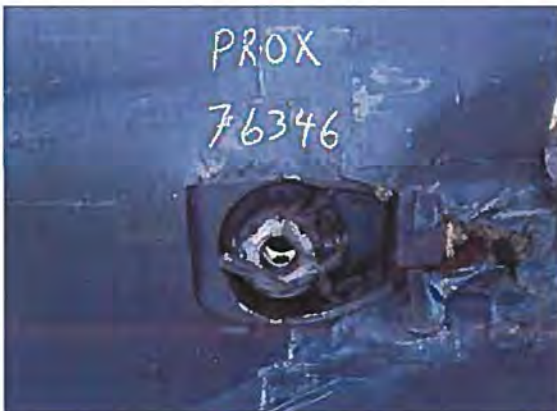
Photo 11. Partially open BOV of car PROX 76346
