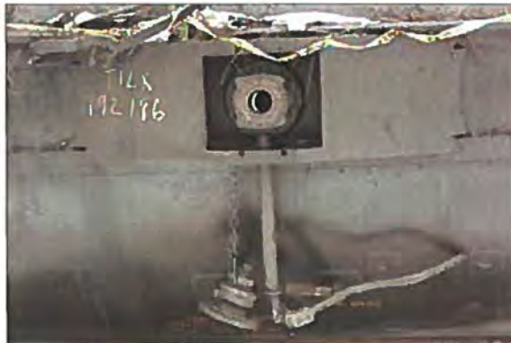
Photo 7. Car TILX 192186 BOV and bent handle
