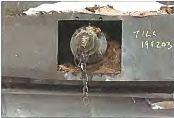
Photo 4. Car TILX 198203 bottom outlet valve (BOV) and skid protection
