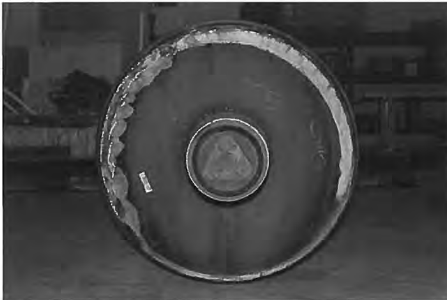
Photo 14. Outboard view depicting the extent of wheel fracture
