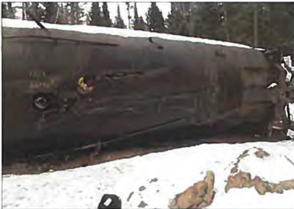
Photo 10. Car PROX 76346 jacket damage
