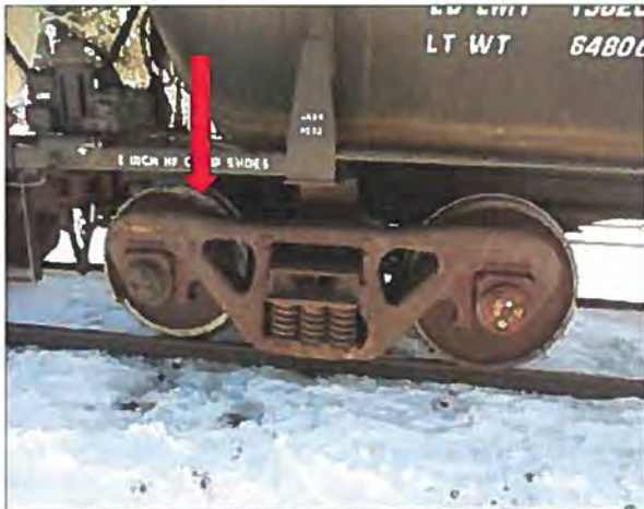
Photo 2. Broken R1 wheel (source: CP Police)
