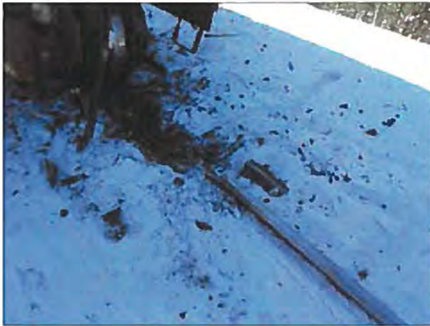
Photo 1. Broken south rail at Mile 9.41 (looking east)
